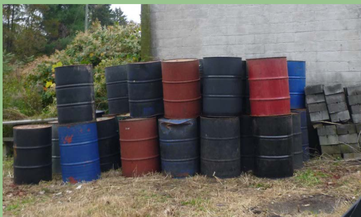
Chemical storage without secondary containment or cover
